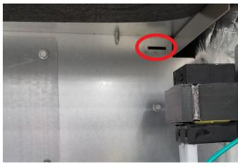
**FIGURE 18. Notch for Control Panel Relocation**
