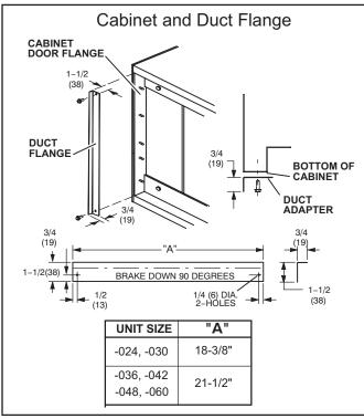
FIGURE 15. Cabinet and Duct Flange
