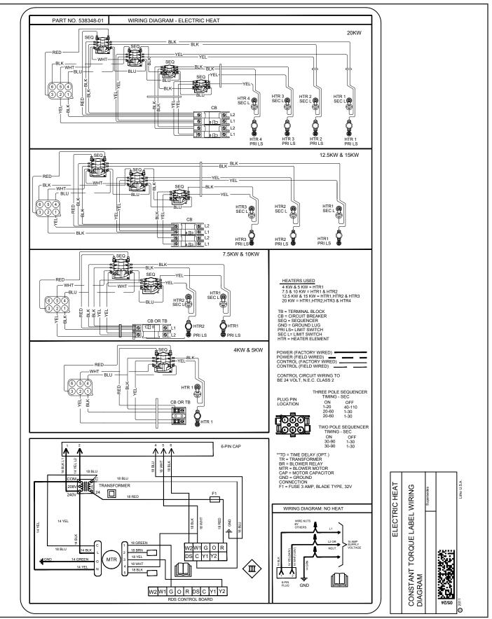
FIGURE 1. Typical Wiring Diagram – HMA\*C\*1S Air Handler with Electric Heat – CT
