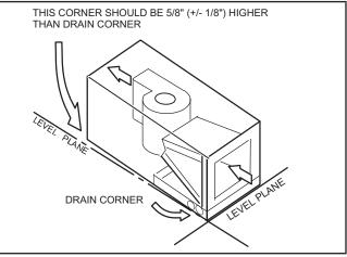
FIGURE 13. Sloping the Unit for Proper Drainage
