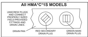
**FIGURE 14. Drain Line Connections**
