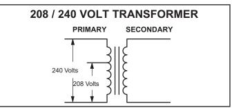
FIGURE 20. Converting Unit from 240VAC to 208VAC
