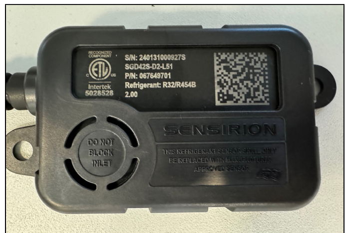
FIGURE 23. Example of Clear, Unobstructed Sensor Inlet
